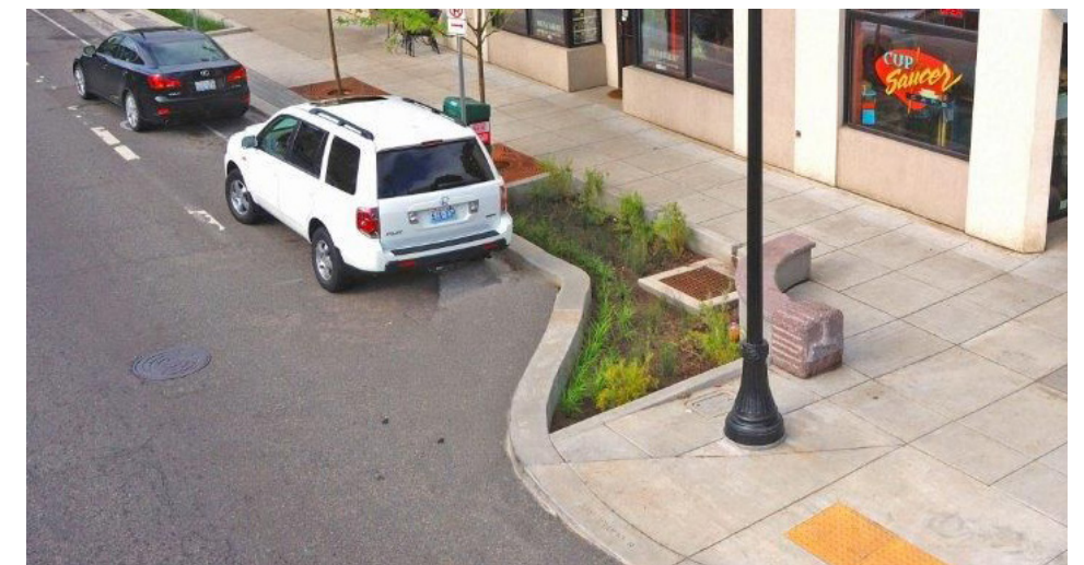
BUMP OUTS CREATE PROTECTED ON-STREET PARKING
